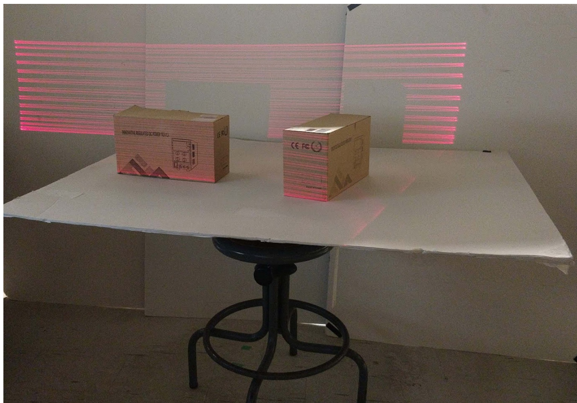
Figure 11. Raster scan pattern (visible laser) with 150 Hz sinusoidal and 5 Hz triangular waves.
