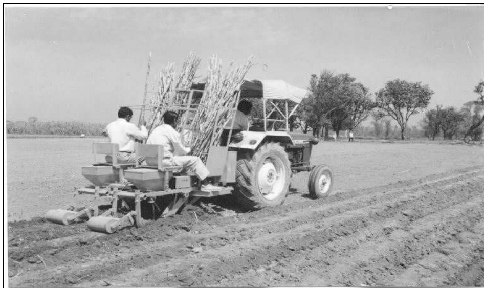
Fig. 2. Two-row tractor operated sugarcane cutter planter
