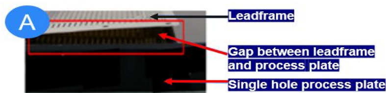
Fig. 1. Gap between the leadframe and the process plate
