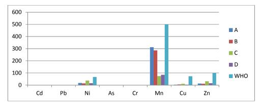
Fig. 3. Concentration of heavy metals in cassava tubers (mg/kg)
