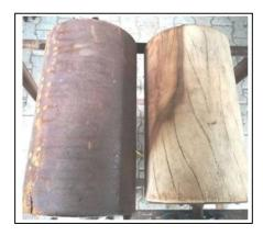
Fig. 2. Threshing mechanism-drive (Wood) and driven (Iron) rollers
