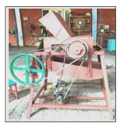
Fig. 3. Power operated portable sesame thresher
